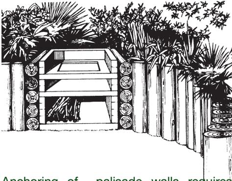
Anchoring of palisade walls requires preparation of a continuous trench with concrete work generally the same as for cantilever walls. Walls taller than 1.2m should slope inward to compensate for any future deflection of the timber or foundations. Staple wire along the tops of logs to provide stability during grouting.
